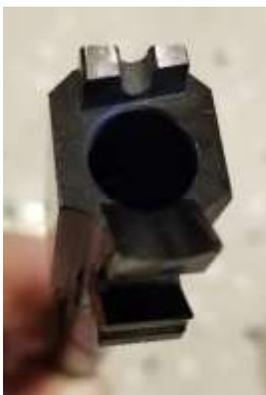
A different fit issue we saw on one of the first 7 slides (from a G2S) we put the threaded barrel in didn't allow the barrel to tilt far enough to allow the longer barrel to drop into place. It required fitting, removing some material along the top front edge and inside
