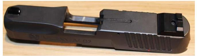
Reassemble the pistol and make sure and allow 24 hours for the thread locker to secure the sights before firing, or even vigorously cycling, the pistol.
