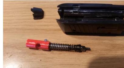
8. A trick for taking the striker assembly apart is to insert it into the striker channel backwards so the spring is easier to compress to remove the keepers. This is also the part you want to be extra sure to have your eye protection on for. Here is how the slide is used to help:
