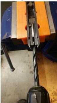
13. Check the fit of the striker in the striker guide. If there is any tightness or binding, adjust the slot width until the striker just moves freely. Reverse the disassembly
