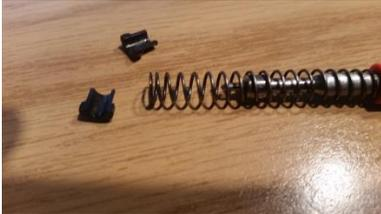
10. If you have a PT111 G2, test whether your striker guide slides in easily past the Taurus Security System cam that is in the striker guide channel. Some will, most will need additional work. If you have clearance and your striker guide slides in easily, skip to step 13. The G2C, G2S, G3, and G3C don't have the TSS and can skip this and the next 2 steps.
