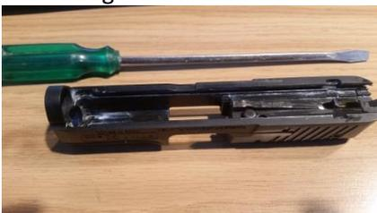
5. To remove the back plate on the slide, the striker guide must be pressed using your tool towards the muzzle and the back plate slides down and out. Here as shown in the photo below:
