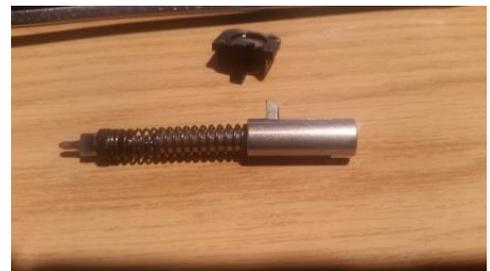
14. Clean everything, the striker assembly, the striker channel, etc. Put the striker assembly into the slide, and depress it using your screwdriver or a punch far enough where you can reinstall the back plate:
