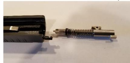
7. A trick for taking the striker assembly apart is to use the slide plate as a spacer to help compress the spring and remove the keepers. This is another area where little parts can go flying and why you want your safety glasses:
