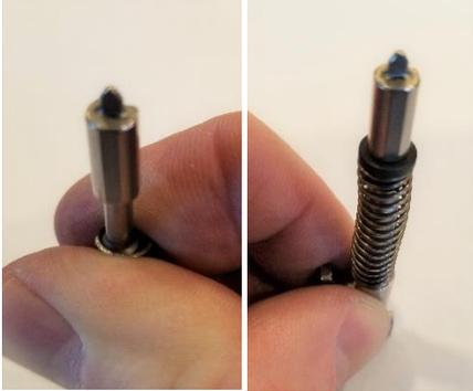
9. Check the fit of the striker in the striker guide. The striker should move freely. There can be some tightness when the end of the striker is out at the end of the slot. It doesn't go there once assembled. Reverse the disassembly process and assemble the striker assembly using the Lakeline striker guide. Here it is ready for the keepers to be installed:
