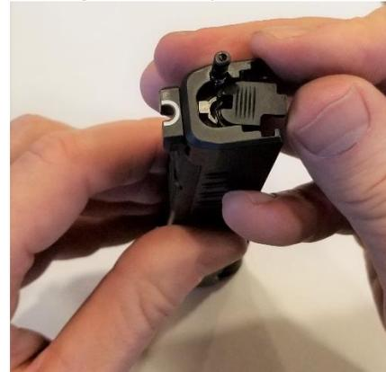
6. Slide the rear plate the rest of the way out and remove the striker assembly:
