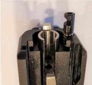
11. Push down the tab on the striker guide, and push in the back plate until it is stopped by
