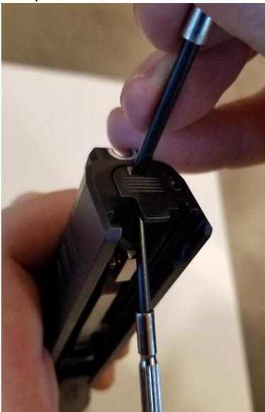
5. After moving the back plate down a little, remove the screwdriver from the tab on the striker guide tab and hold your thumb over the extractor spring retainer. This is important so it doesn't go flying.
