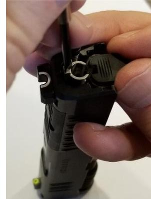
12. Now, take a small screwdriver and push down the extractor retainer until the slide plate can be pushed up all the way and snap into place. It takes some pressure to push the extractor retainer down, the spring is stiff:
