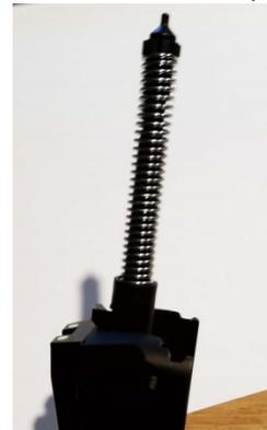
8. When you compress the spring from the top (muzzle end) of the striker, the keepers can be slid out each side. You can see how the keeper works from the disassembled striker below:
