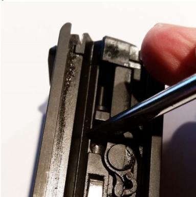
6. Remove the back plate, and then the striker assembly, so you have your assembly like like this:
