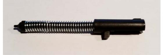
7. A trick for taking the striker assembly apart is to insert it into the striker channel backwards so the spring is easier to compress to remove the keepers. This is also the part you want to be extra sure to have your eye protection on for. Here is how the slide is used to help:
