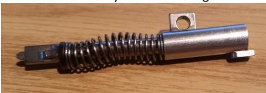
12. When putting the striker assembly into the slide, it may take some jiggling and aligning of the spring to get it to go in far enough where you can reinstall the back plate. It should slide to this point without compressing the spring to be ready for the
