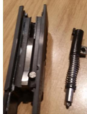
8. A trick for taking the striker assembly apart is to use the back plate under the striker tab so the spring is easier to compress to remove the keeper. I also set it on something on my desk or bench so it won't slide, like a piece of paper or tablet. This is also the part you want to be extra sure to have your eye protection on for. Here is how the rear plate is used:
