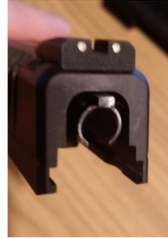
10. Clean everything, and reassemble using the Lakeline Striker Guide. In this photo I am preparing to reinstall the striker spring:
