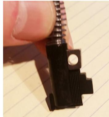
9. When you compress the spring from the top (muzzle end) of the striker, the keeper can be slid out to the side. You can see how the keeper works from the disassembled
