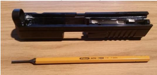
5. To remove the back plate on the slide, the tab must be pressed using your tool and the back plate slides down and out. Here is the tab to press:
