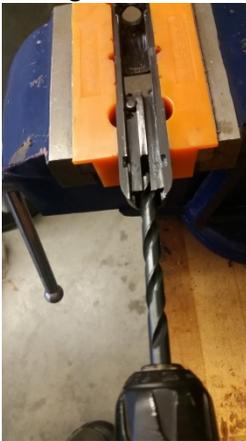
13. Check the fit of the striker in the striker guide. If there is any tightness or binding, adjust the slot width until the striker just moves freely. Reverse the disassembly process and assemble the striker assembly
