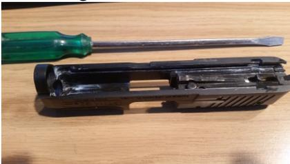
5. To remove the back plate on the slide, the striker guide must be pressed using your tool towards the muzzle and the back plate
