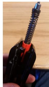
9. When you compress the spring from the top (muzzle end) of the striker, the keepers can be slid out each side. You can see how the keeper works from the disassembled
