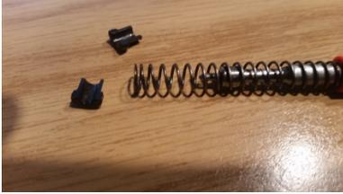
10. Test whether your striker guide slides in easily past the Taurus Security System cam that is in the striker guide channel. Some will, most will need additional work. If you have clearance and your striker guide slides in easily, skip to step 13.
