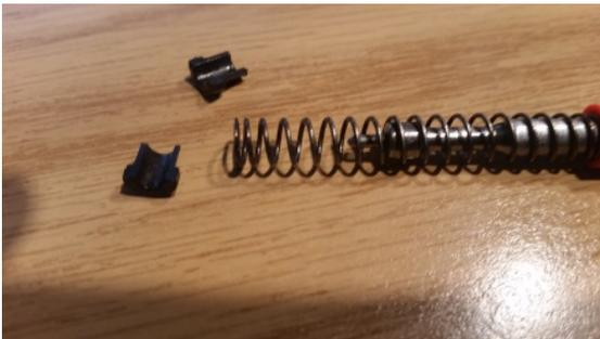
10. Replace both springs. Both springs should be replaced at the same time. Reverse the disassembly process and assemble the striker assembly:
