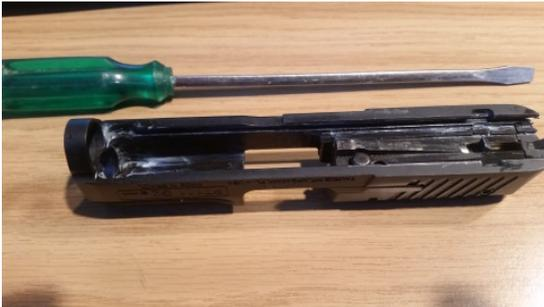
5. To remove the back plate on the slide, the striker guide must be pressed using your tool towards the muzzle and the back plate slides down and out. Here as shown in the
