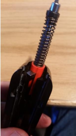
9. When you compress the spring from the top (muzzle end) of the striker, the keepers can be slid out each side. You can see how the keeper works from the disassembled striker below:
