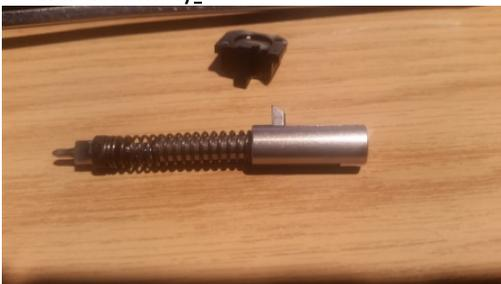
11. Clean everything, the striker assembly, the striker channel, etc. Put the striker assembly into the slide, and depress it using your screwdriver or a punch far enough where you can reinstall the back plate:
