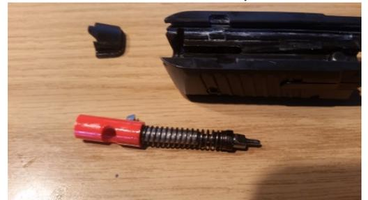
8. A trick for taking the striker assembly apart is to insert it into the striker channel backwards so the spring is easier to compress to remove the keepers. This is also the part you want to be extra sure to have your eye protection on for. Here is
