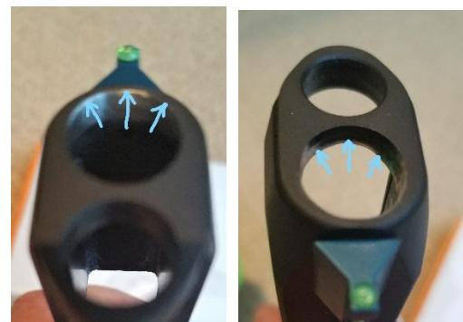
**If it isn't clear to you, don't do it.** A gunsmith can fit it for you. It takes a little hand work with a round file, cleaning up the file marks, and refinishing the edges with some cold blue on a black slide. Done properly, the barrel will still lock up as accurately as before.
