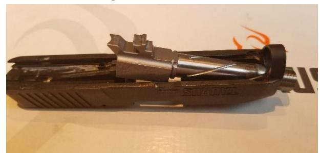
Material needs to be removed from these 2 edges to allow the barrel to tip a little further so it can be slid in:
