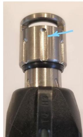
The o-ring allows the port to be aligned and it can be compressed enough to keep tension on the threads so the compensator stays clocked into proper alignment. If desired, some low strength (green) thread locker can also be used in addition to the o-ring.
