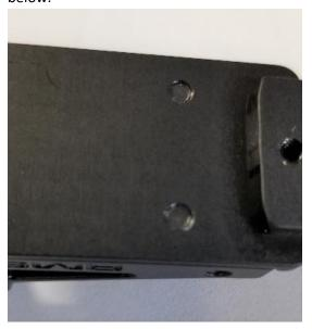
You will still be able to remove the screws and lift the Romeo O out to change batteries with the shortened bosses.
