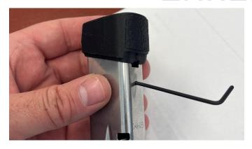
Remove the allen wrench and the spring will lock into place.
