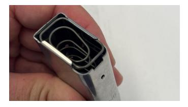
Using needle nose pliers or hemostats, clamp on the front of the spring and push in toward the top of the magazine to compress the spring. Once in, slide the allen wrench in to hold the spring in a compressed position.
