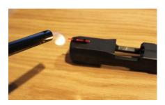
Reassemble the pistol and make sure and allow 24 hours for the thread locker to secure the sights before firing, or even vigorously cycling, the pistol.
