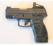
**ROMEO 0 SHROUD:** The Romeo 0 shroud is heavy and acts like a guillotine to the bosses on the sight mount plate, and will cut them off, if you do not do these additional steps: The bosses on the top of the plate have to be filed down to 0.10 inch in height. Thread locker needs to be liberally applied between the shroud and the mount plate. As in the earlier instructions, use screws that extend to the bottom of the plate and don't over tighten them.
