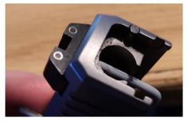
• Carefully remove coat hanger tool while containing the striker spring and plunger. It will fly, so be careful. The extractor plunger will also fall out from gravity if you don't keep it in place as well:
