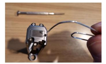
• The plunger you are depressing looks like this with the back plate removed:
