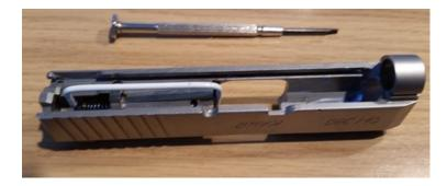
• Use modified large paper clip, rod, punch and depress extractor spring plunger so back plate can be slid off:
