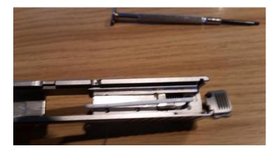
By depressing the firing pin block, sometimes a couple of times, you should be able to slide out the striker and spacer. The Lakeline Striker and Spacer is a matched set and the spacers CANNOT be interchanged with the factory part. Your pistol may be unsafe or inoperable if you interchange them. The Lakeline parts are on the left in the photo below:
