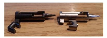
• Install the Lakeline Ultimate Striker and Spacer and reverse the disassembly process to reassemble. The striker spring can send itself and the plunger flying, so be careful.
